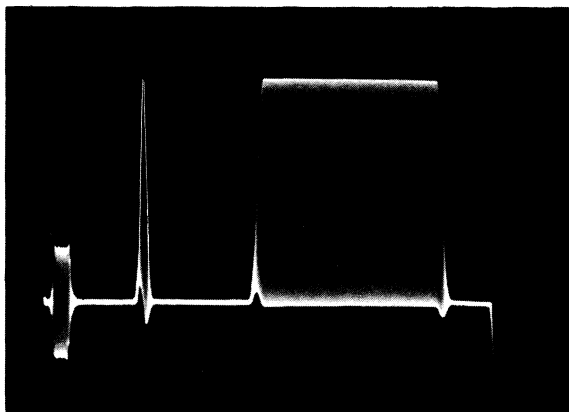
Fig. 9. Delay inequality indicated by the combined luminance and chrominance sine squared pulse and bar.
